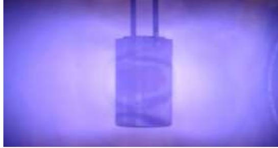
**Figure 3.** Digital picture of Argon plasma in the dipole magnetic field, at a neutral pressure of 0.2 mTorr and microwave power of 300 Watt.
